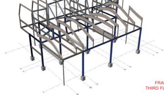
BRACED FRAME THIRD FLOOR
